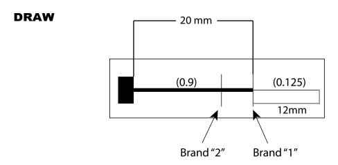
The connector kit incorporates a polished fiber section of the factory with a mechanical splice and the body of the connector
